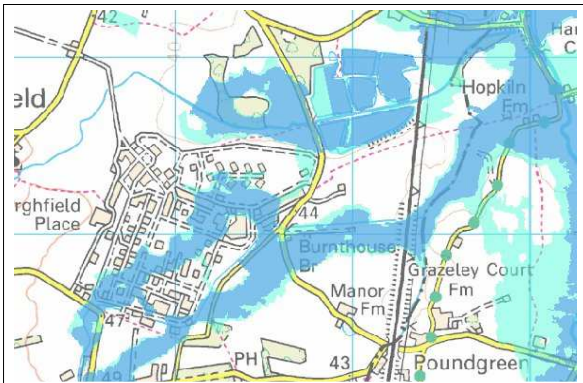
Figure 1. Flood map for AWE Burghfield 3 . Shaded areas represent areas at significant risk of flooding, where the chance of flooding each year is greater than 1.3% (1 in 75).
