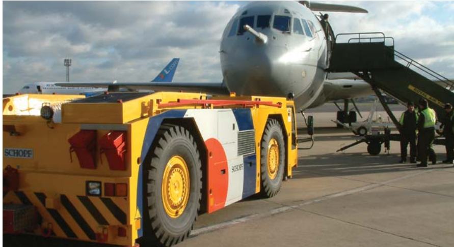
Give me strength: the new aircraft tow tractors that can pull the biggest aircraft in the world
