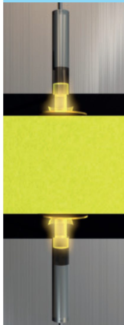
A section of the test assembly, showing the probe configurations.
