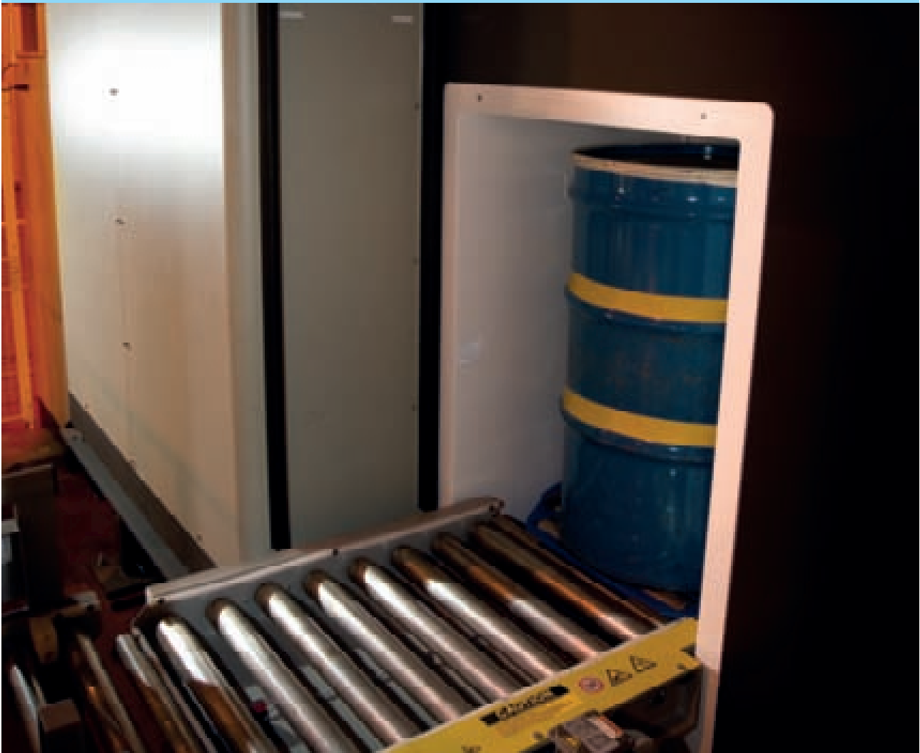
The installed SILWAS system showing the conveyor linkage between the two assay elements, the AQ2 and the HENC. Figure shows a drum inside the HENC component of SILWAS.
