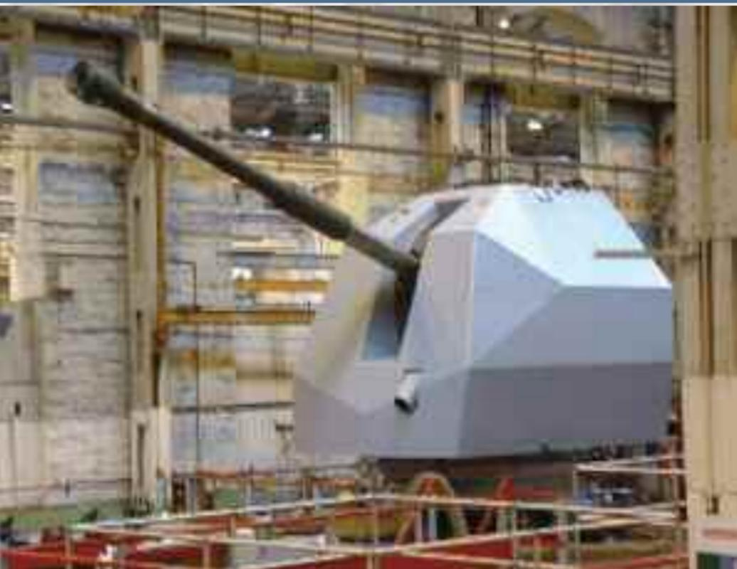
**BAE Global Combat Systems have designed and built a prototype 155mm naval gun. It should be retrofitted to Type 23 and Type 45 warships and incorporated into the planned Type 26 Future Surface Combatant.**
