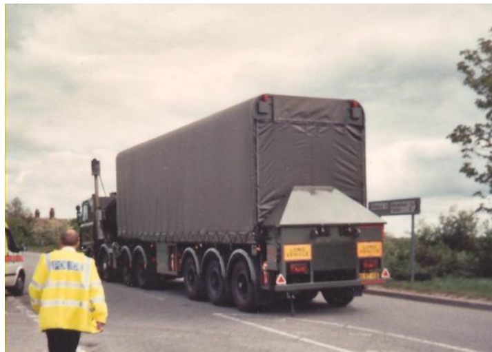
Photograph 1 Rear of an Articulated Vehicle – Note the full height and width of the trailer unit obscuring the forward view to a vehicle behind
