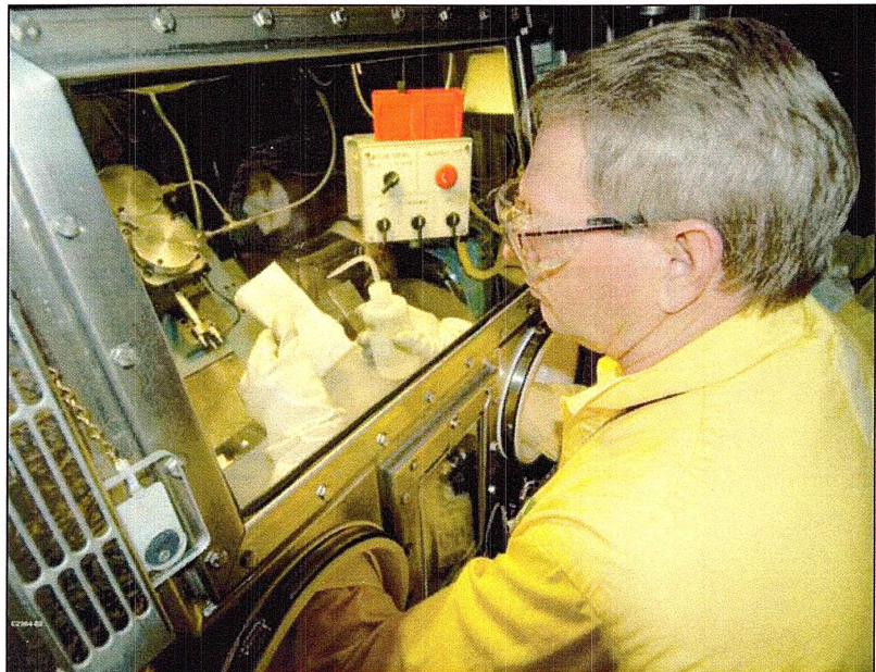
Literally taking thousands of hours to make, the use of Plutonium in Pit Manufacturing requires the specialized skills of a glovebox worker to cast, shape, inspect, and assemble the needed components into quality product.
