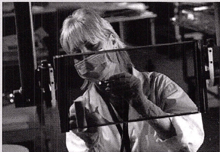
Inspection of the first batch of Orion laser glass (Photo courtesy of Zygo Corporation)
