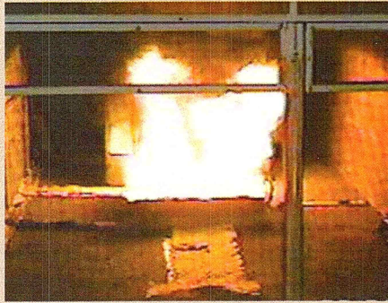
W76-1 re-entry body qualification test in wind-driven pool fire
