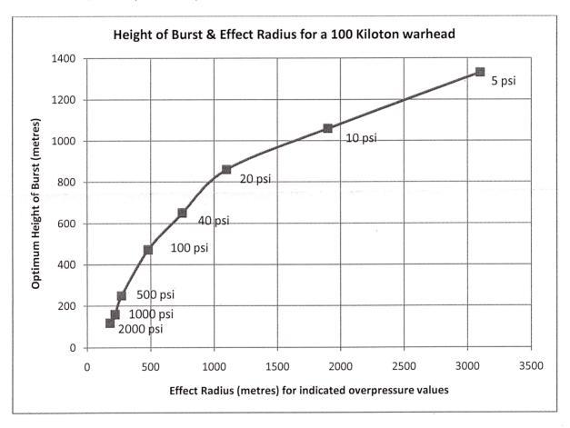
The chart shows the effect radius for various overpressures and the optimum height of burst associated with this overpressure for a 100 kiloton warhead.
