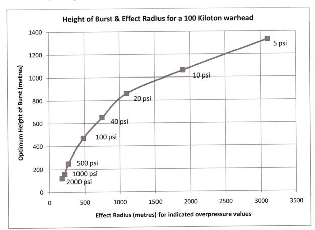
The chart shows the effect radius for various overpressures and the optimum height of burst associated with this overpressure for a 100 kiloton warhead. <sup>5</sup>
