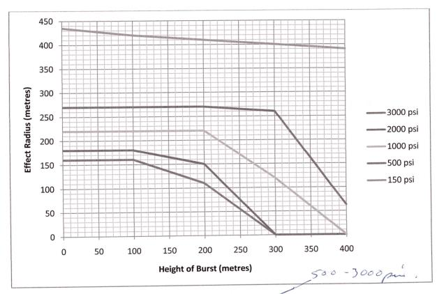
The chart shows the effect radius for different psi values if a 100 kiloton warhead is detonated at different heights. It illustrates the range of hard targets that might be attacked with a near surface burst capability on the Mk4A. This would allow the warhead to be detonated closer to the ground than the fireball radius of around 250 metres. It suggests that to be effective against targets in the 2000 – 3000 psi range the Height of Burst would have to be lowered to 100 metres.
