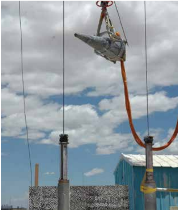
W88 warhead undergoing a drop test as part of the Alt-370 Life Extension.
