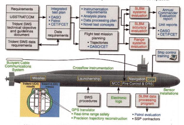
SSD contributes to the continuing Navy Fleet Ballistic Missile Strategic Weapon System test and evaluation programs. (SSD-developed hardware, green; documents/reports, blue; programs, red. MCC = missile control center, DRS = Data Recording System, DRN = DASO Reference Navigator.)
