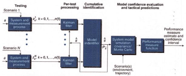
Strategic Weapon System accuracy evaluation concept,  $\theta = \text{model parameter}$ ,  $\hat{g} = \text{estimate of parameters derived from tests}$ ,  $P_{\hat{g}} = \text{estimation error covariance matrix}$ ,  $Z_k^j = \text{measurement } k \text{ from test } j$ .
