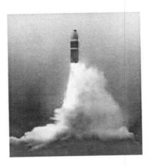
**Description:** The TRIDENT II (D-5) is a submarine launched ballistic missile with greater range, payload capability and accuracy than the TRIDENT I. The major contractor is Lockheed Martin Missiles and Space Company, Sunnyvale, CA.
