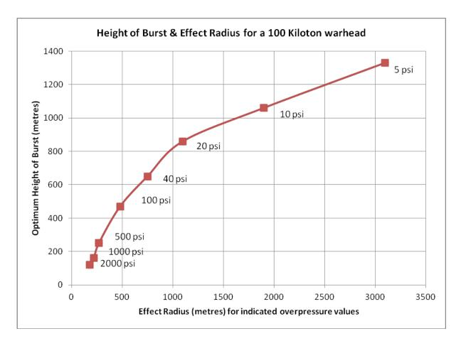
The chart gives a general indication of how the optimum height of burst varies with the intended blast effect. It shows the effect radius for various overpressures and the optimum height of burst associated with this overpressure for a 100 kiloton warhead.<sup>5</sup> This illustrates how both greater accuracy and a lower Height of burst are required to attack harder targets.
