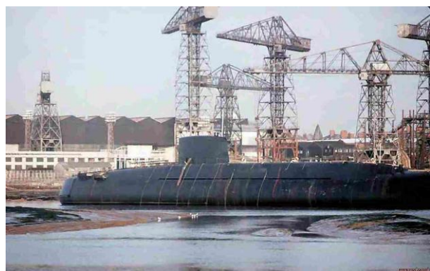
HMS Repulse in Walney Channel in 1965. The Polaris submarine ran aground after being launched. The extensive sandbanks around Barrow are one reason why the site would not become an operational base.
