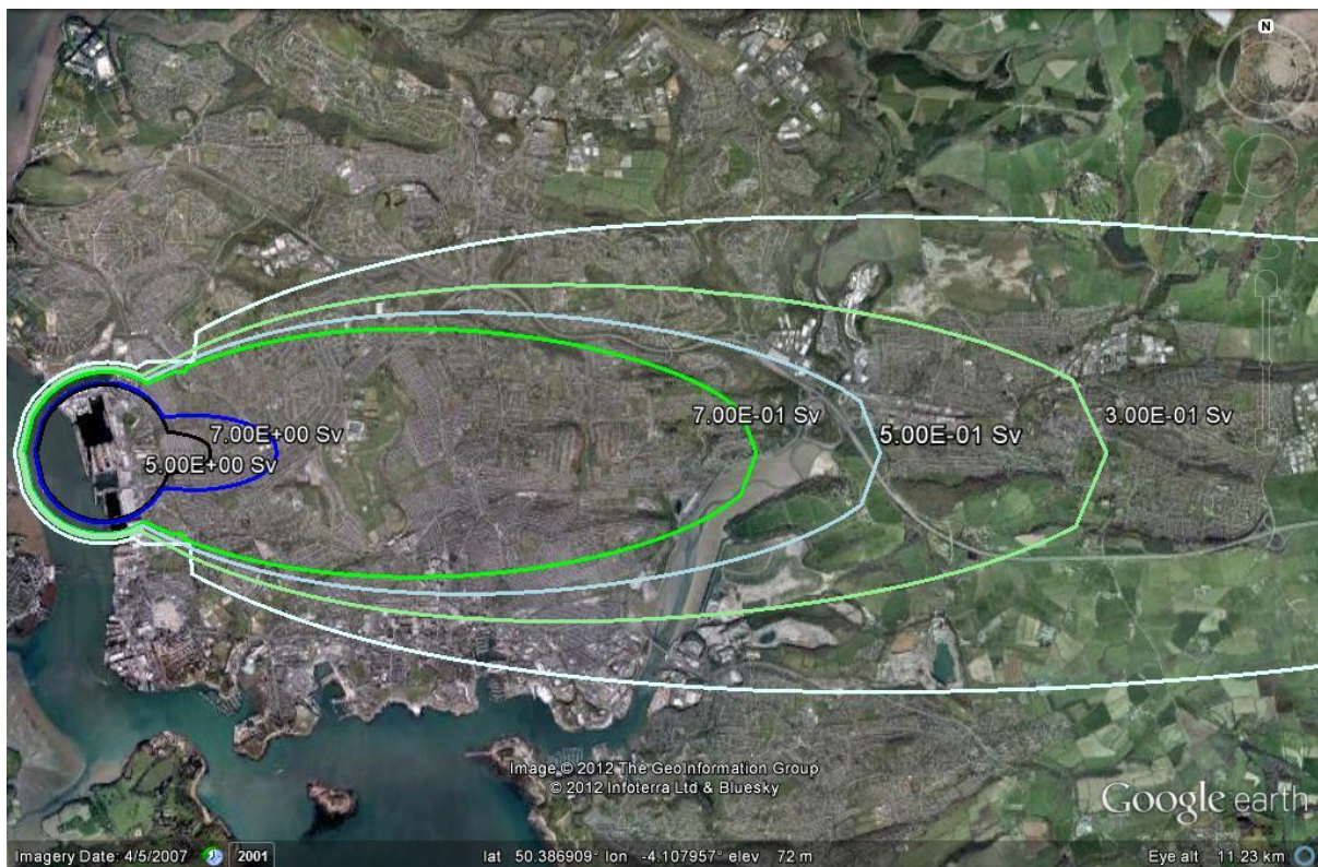
Map 4. Total Effective Dose Equivalent after 24 hours windspeed 0.1 m/s stability A from West
