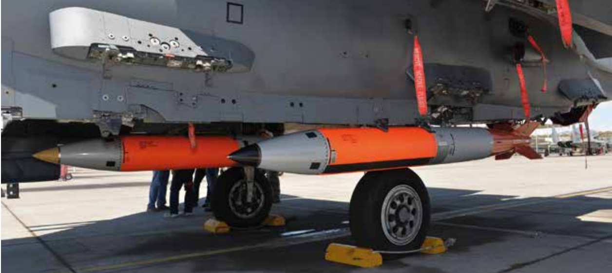
Two B61-12 development shapes (Joint Test Assembly) under F-15E during test flight in 2015.
